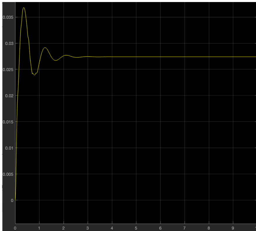
Figure 14, showing damping and eventual equilibrium of sinkage
